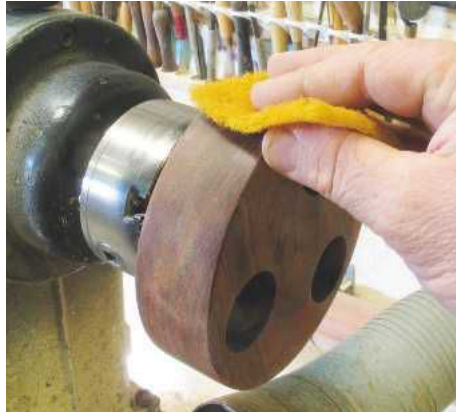
▲ Pic.14 Cut back the sealer with 0000-grade wire wool or use the Nyweb equivalent as here, which won't leave metal dust like wire wool can and is also much safer around grinders etc
